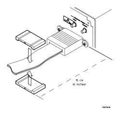
**2** Insert the clamps onto the ends of the ferrites. The locking tab should fit cleanly in the ferrite grooves.
