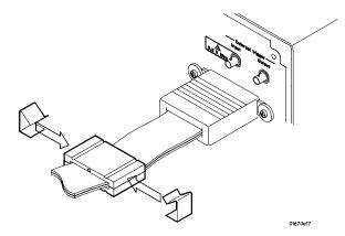
When properly installed, the ferrite should appear on the logic analyzer cable as shown.
